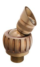
Micro-directional luminaire with solid brass construction, features a Thermally Integrated® LED module and interchangeable acrylic optics. The easily replaceable, self-contained ball fits snugly into a precision machined socket for exceptional heat dissipation. Offered in 4 unique shroud configurations. Available as stake, flush, or surface mount. Downlight version also available.
